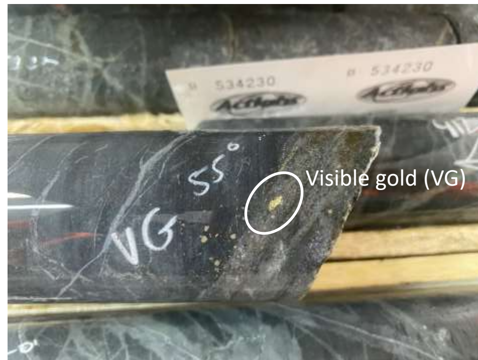
Hole FG21-158: Photo showing a visible fleck of gold at 411.9m. Assays pending.
